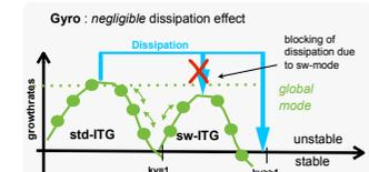
We conclude that the appearance of the sw-ITG mode blocks the dissipation of std-ITG mode thus the stabilization effect of a magnetic island on ITG waves is reduced.
