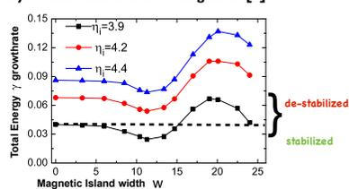
Stabilization effect due to mode coupling and dissipation of energy by stable modes
