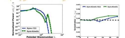
(The sw-ITG mode can be clearly seen in the turbulence spectra (picture left). The dependence of total energy growth vs. Island size w with sw-ITG mode shows very weak stabilization effects. Destabilization dominates with island size bigger than w=8 (picture right)
