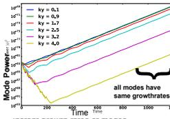
Poloidal coupling leads to the formation of a global mode (all modes have same frequency and growthrate). Energy can be transferred from unstable modes to stable modes and dissipated by away.
